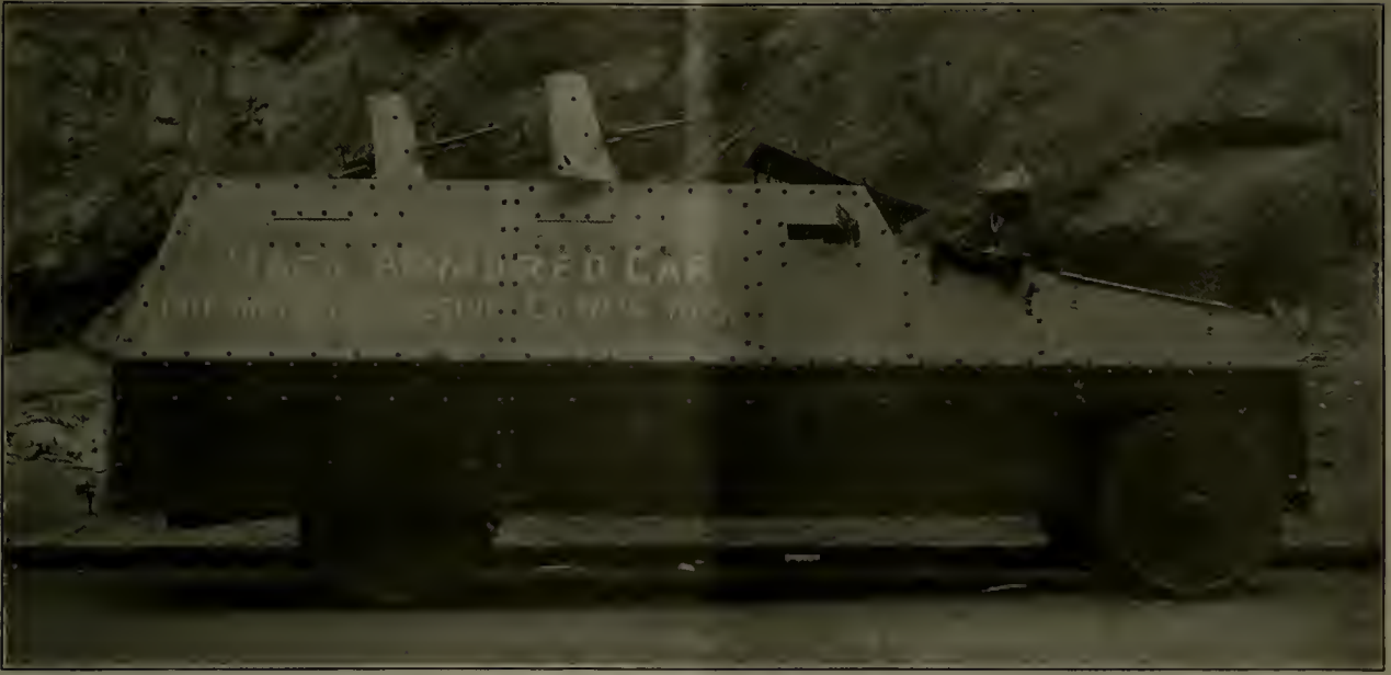
Mack armored car, equipped with automatic machine guns. Used by the National Guard of New York
